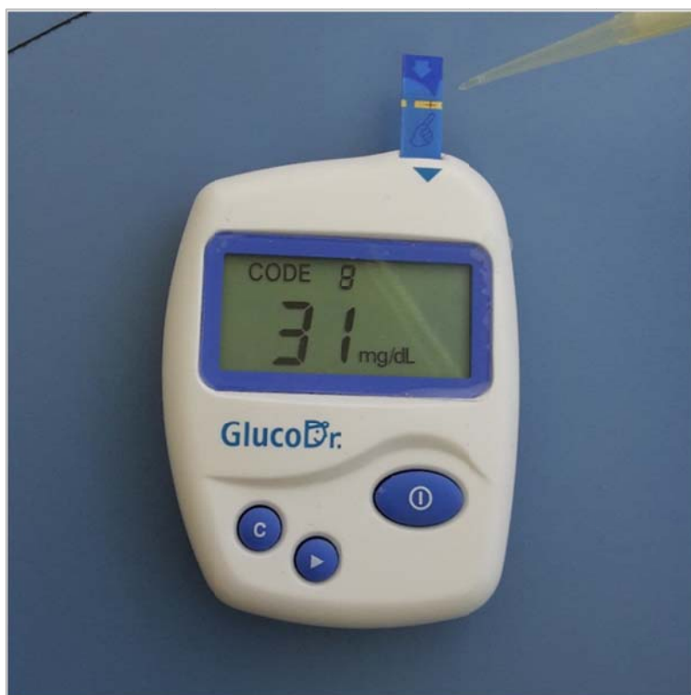
Plate 3 The Glucometer™ showing the sugar concentration (glucose) reading of one of the flowers with the Glucometer™ Strip inserted (blue strip on the top). The pointer shows where the nectar was placed.
