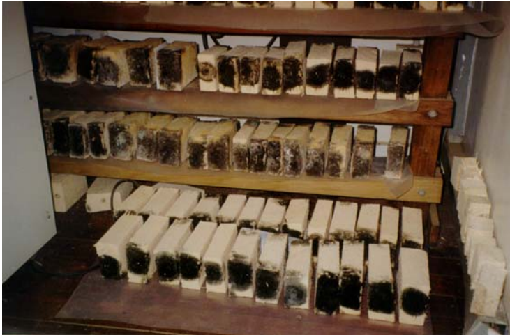
Figure 17. Oil palm wood blocks in plastic bags one day after being inoculated with Ceratocystis cultures.
