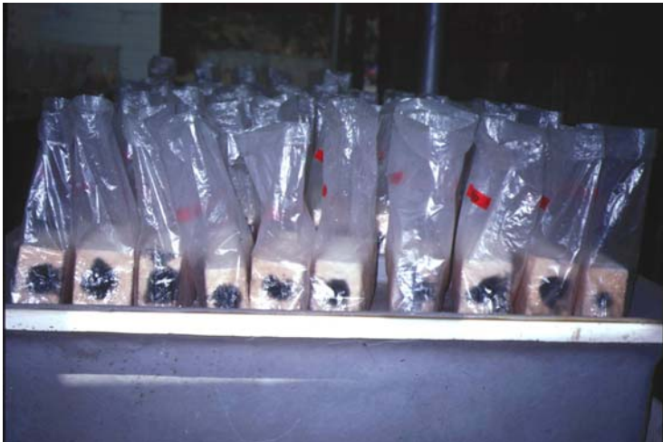
Figure 19. Wood blocks being dried after seven days to check shrinkage due to degradation by Ceratocystis .
