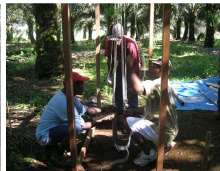
Figure 5. Using pulley to winch out core
