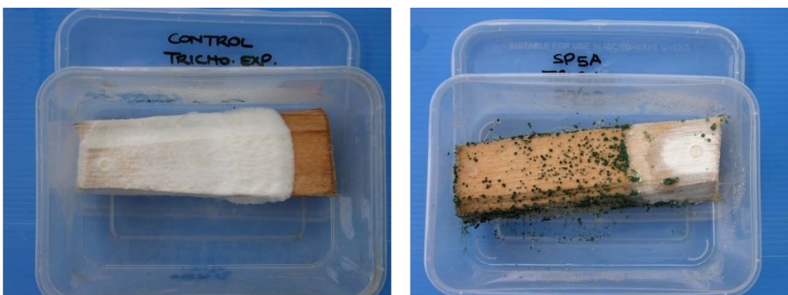
Figure 2.2 Suppression of the growth of a Ganoderma mycelial culture by Trichoderma culture SP5A on oil palm rachis. On the left is the control.
