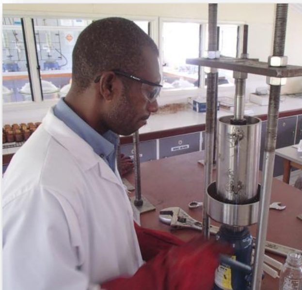
Plate 3 Laboratory-scale CPO extraction device in operation during the extraction process.
